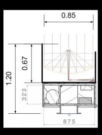
Mass ~250 kg (S/C + payload) assuming SiC mirror @25 kg/m<sup>2</sup>
